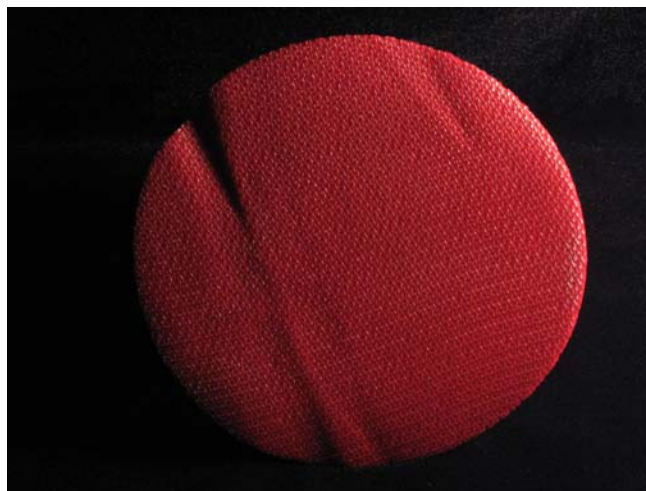
Photo 11: Wrinkle Example - Lava Cloth™ has memory. This piece of Lava Cloth™ had a crease in it before it was pre-fired. The crease remained after pre-firing and the 5", two layer circle was then fired on the cloth. Lava Cloth™ should be stored and shipped flat or rolled up to avoid wrinkles.
