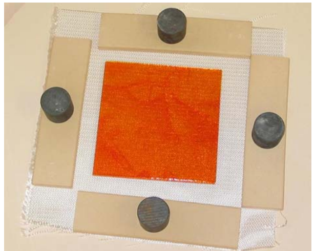
Photo 10: A typical weighting arrangement for a piece of Lava Cloth™. Stainless steel weights on top of Hot Damz arranged around the edge of the cloth.
